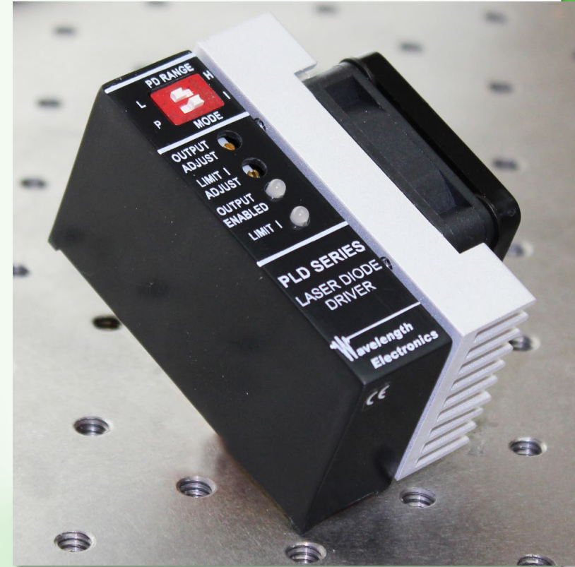
Size (PLD200/500): 1.5 x 2.7 x 0.8 in (39 x 67 x 21 mm) (PLD1250/5000/6500): 1.5 x 2.7 x 1.8 in (39 x 67 x 45 mm)
